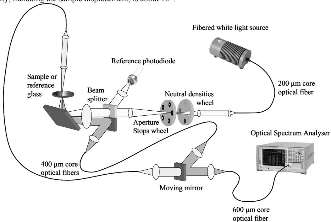
Figure 1. Schematic representation of the spectrophotometer. Calibrated apertures permit to define on the sample a probing zone diameter from 100  $\mu\text{m}$  to 2000  $\mu\text{m}$ . Spectral range extends from 400 to 1700 nm and resolution from 0.5 to 5 nm
