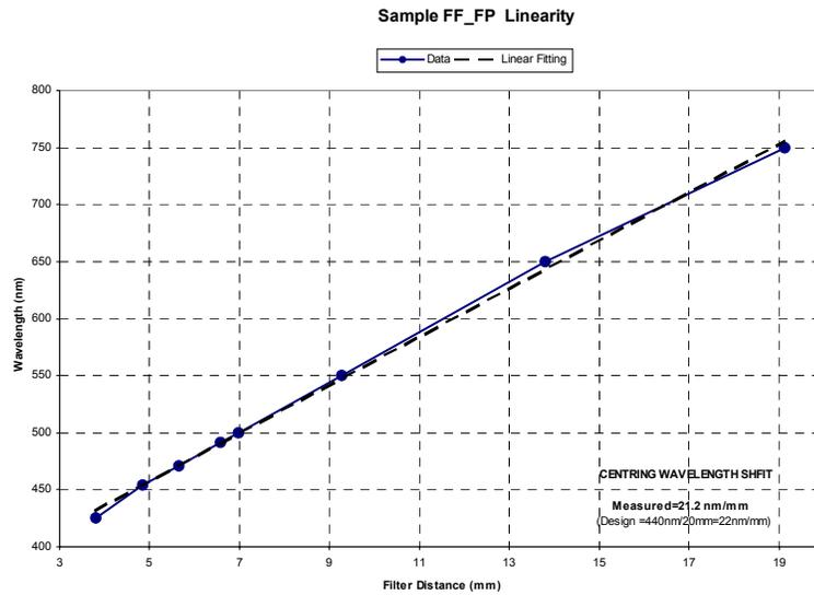
Figure 7. FF\_FP peak transmittance wavelength shift, measured with the CCD-based setup: the measurement data (solid line) and its linear fitting (dashed line)
