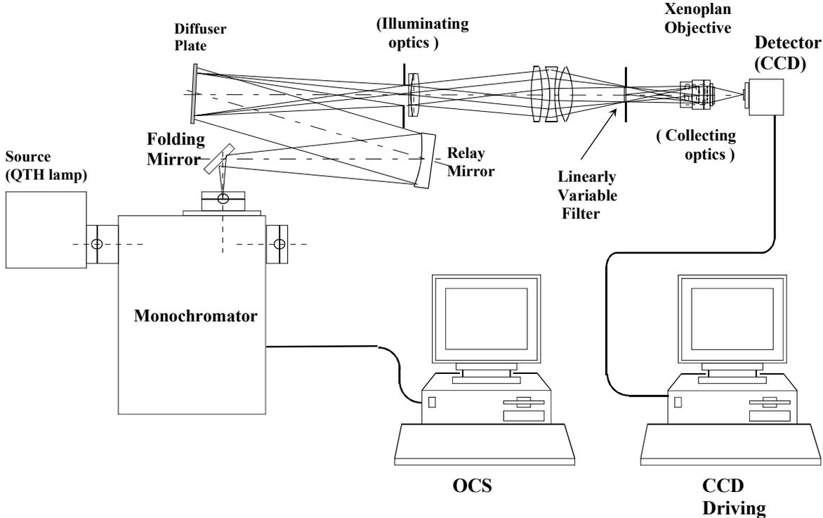
Figure 2. Schematic representation of the CCD-based optical bench
