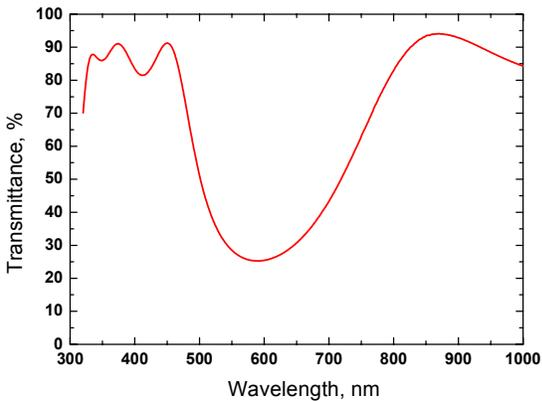
Figure 8. Sample G5TS37: transmittance measured at the point of the maximum coating thickness
